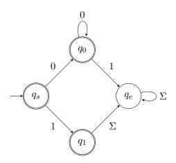
This DFA has four states, but by inspection, we can see that any string  $s \in L(M)$  must enter a loop after the second character. To summarize, |Q| need not be equal to p; it is simply an upper bound.
