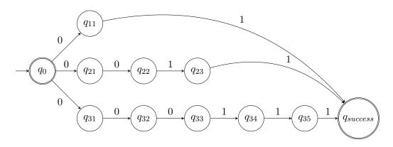
Even with an NFA, it's still clear that this machine grows pretty quickly as well. Each increase in n requires the addition of another branch, which is 2n - 1 states in length. Unlike the first one, however, that this isn't a minimal DFA, so we could potentially grow by a smaller amount, but the important thing to note is that a finite automaton for this language grows proportionally to the upper bound on n.
